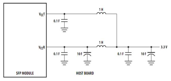
\* Inductors must have less than 1 series resistance to limit voltage drop to the SFP module
